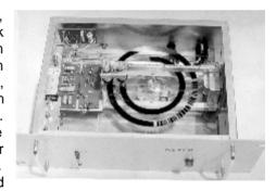
carrier, followed by 15 seconds of tone amplitude modulated on the carrier, then another 15 seconds of unmodulated carrier, then the callsign sent by keying the carrier, before repeating the sequence. The keyer unit was self contained with its own internal power supply.
