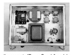
This beacon was a hybrid design (incorporating a transistorised Tx exciter and keyer plus part of the power supply, and thermionic valves
