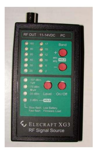
The scribe picked up a small Elecraft XG3 signal generator which uses a PLL IC and attenuation to give set levels (1 uV, 50 uV, 5mV and 223mV (0 dBm) for most amateur bands to 144 MHz. Runs on a PP3 9V battery and fits with my other portable kit.
